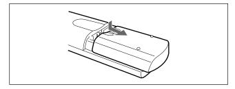
2. Insert two size AA (R6) batteries (supplied) with correct polarities into the battery compartment.
